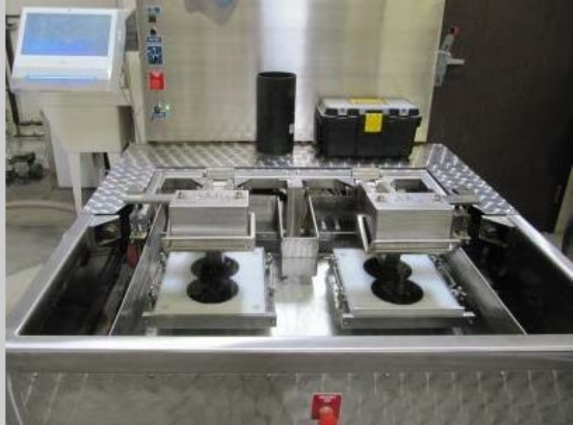
A Hamburg Wheel Track device.
