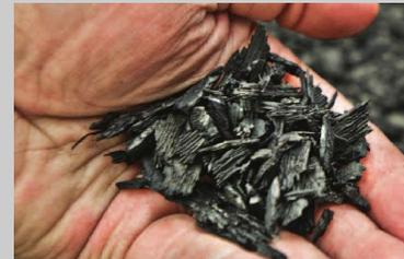
***Processed crumb rubber ready for use in asphalt pavement mixes.***
