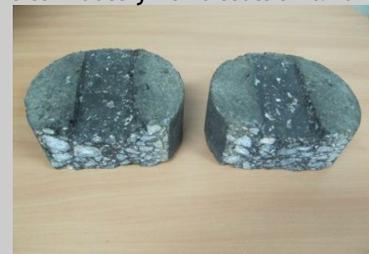
***Samples from a Hamburg Wheel Track test.***
