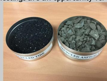
*A sample of Reclaimed Asphalt Pavement (RAP) is on the right, next to a sample of crumb rubber.*
